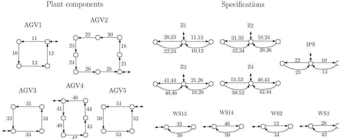
Fig. 15. Generators of plant components and specifications.
